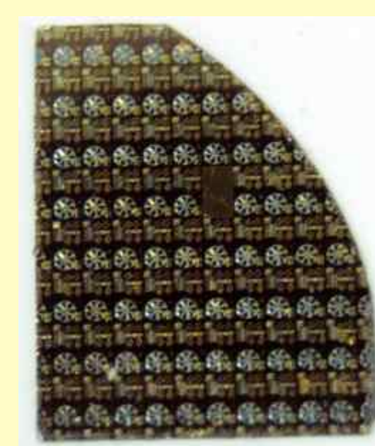
GaAs wafer with fabricated photovoltaic structures
